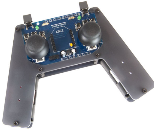
Figure 3.16 The hand-held remote called ArbotiX Commander. It provides 6 buttons, 2 trigger buttons and 2 joysticks.
