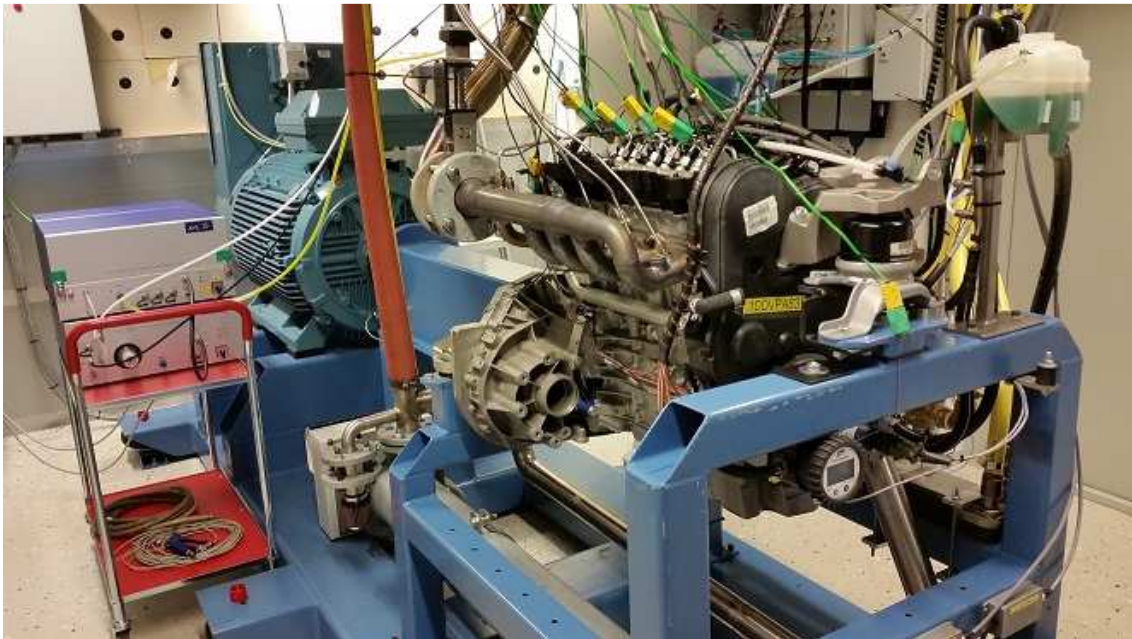
Figure 3.1: Volvo lab engine. Diesel-CNG Dual Fuel Engine
