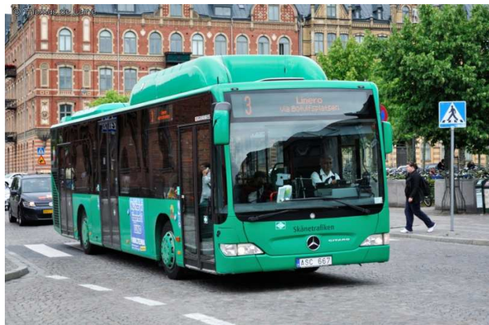
Figure 2.8: A CNG powered Mercedes-Benz O530 Citaro bus, operated by Bergkvarabuss in Lund, Sweden.
