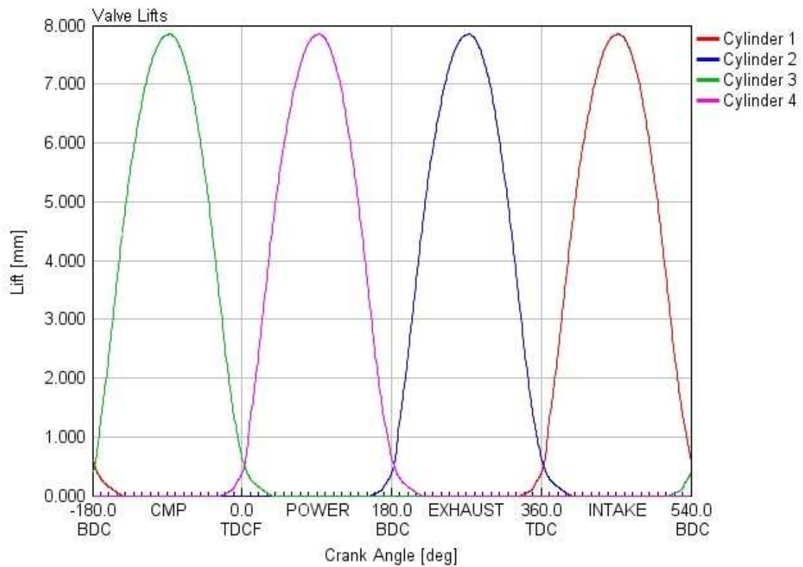
Figure 4.21: Intake valve lifts
