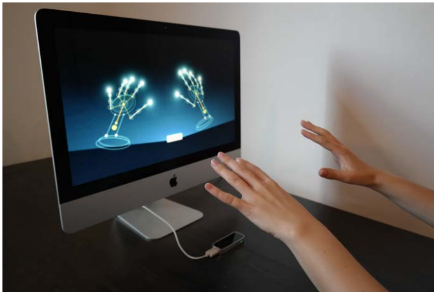
Figure 2.2: The figure illustrates how a user's hands are realized on a screen when using the Leap Motion-technology (VJs Mag 2015).
