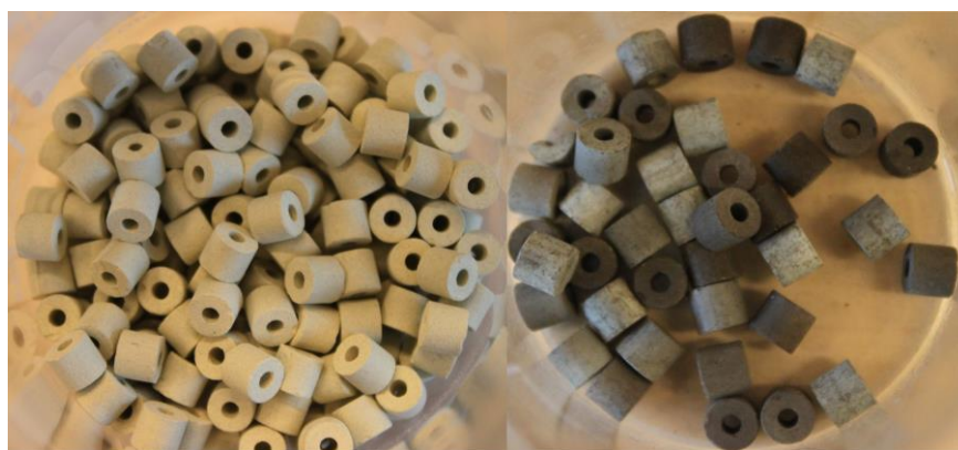
Figure 5.13. On the left an unused catalyst can be seen and on the right a used catalyst.
