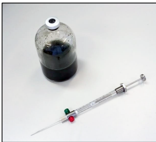
Figure 3.7. Bottle used in BMP tests and the glass syringe used for collection of gas samples.
