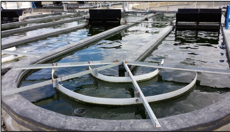
Figure 2.2. Pilot scale raceway pond for treatment of wastewater using algae, in Spain (picture taken by Lars-Erik Olsson, AnoxKaldnes).
