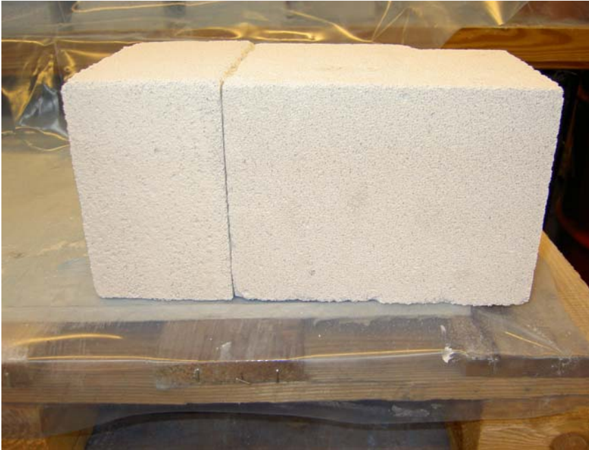
Figure 13. The two blocks joined with mortar.
