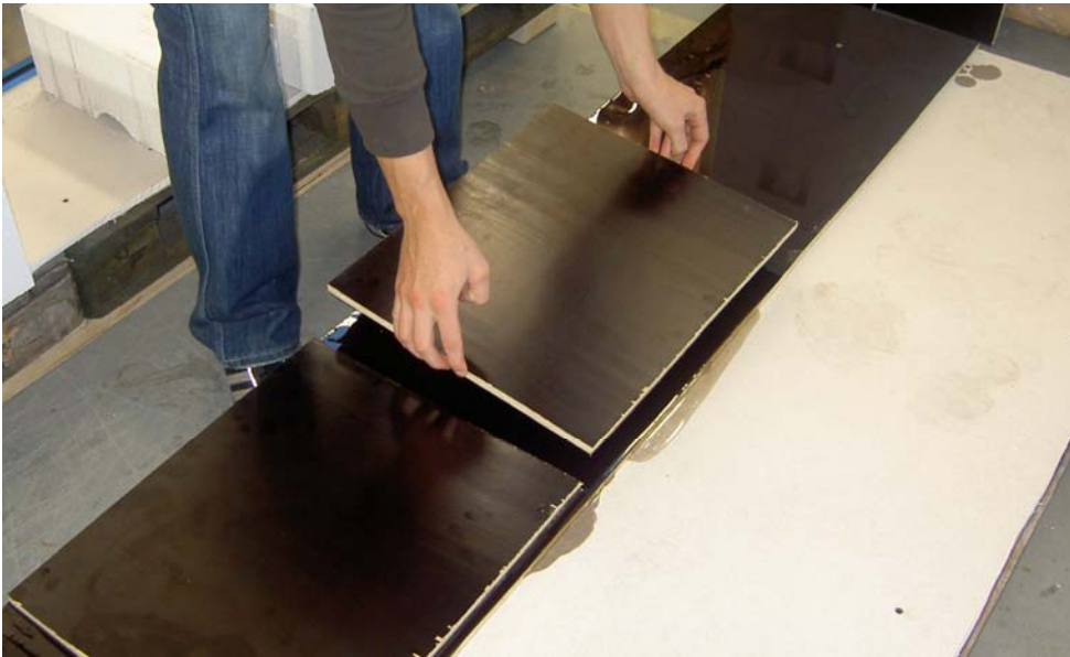
Figure 5. Plywood with oil in between in order to reduce friction.
