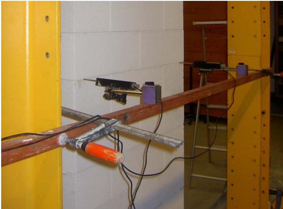
Figure 9. Deflection gauges fitted on the masonry- flexural strength.
