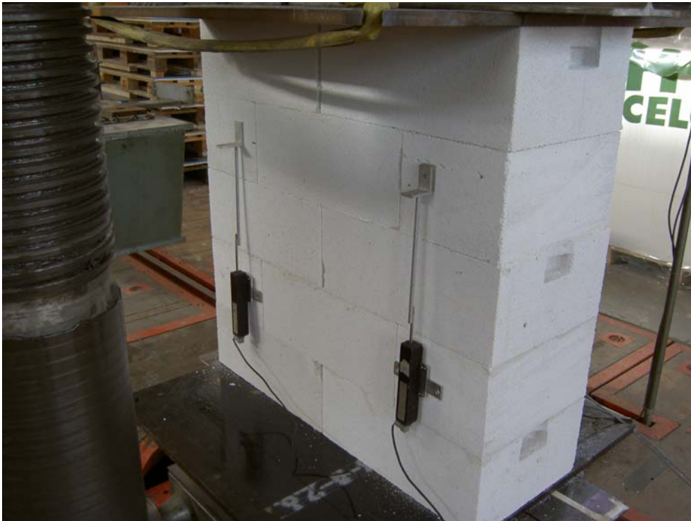
Figure 12. Deflection gauges attached to the masonry- compressive strength.
