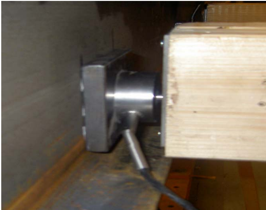
Figure 8. Load indicators between strut and beam.
