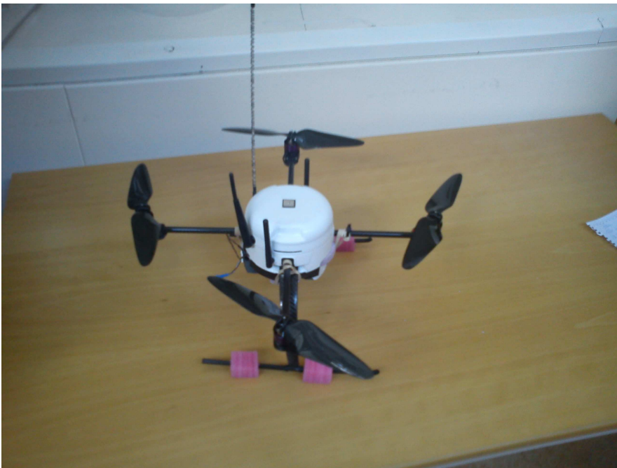
Figure A.2: Top view of the repaired LinkQuad after a crash from 5 m above the ground.
