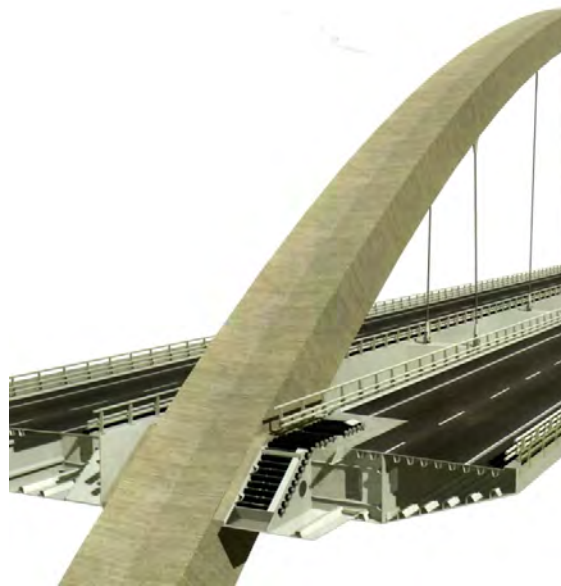
Figure 11 - Connection between the steel superstructure and the concrete arch rib
