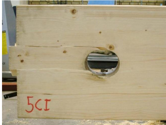
Figure 48 Typical failure mode: shear plug.
