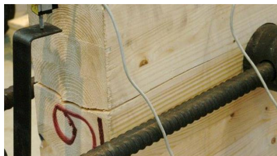
Figure 36 Splitting in specimen 9.
