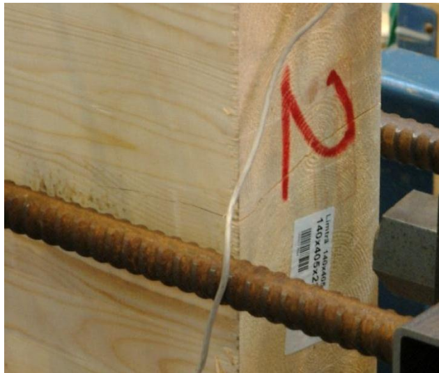
Figure 28 Splitting in Specimen 2.
