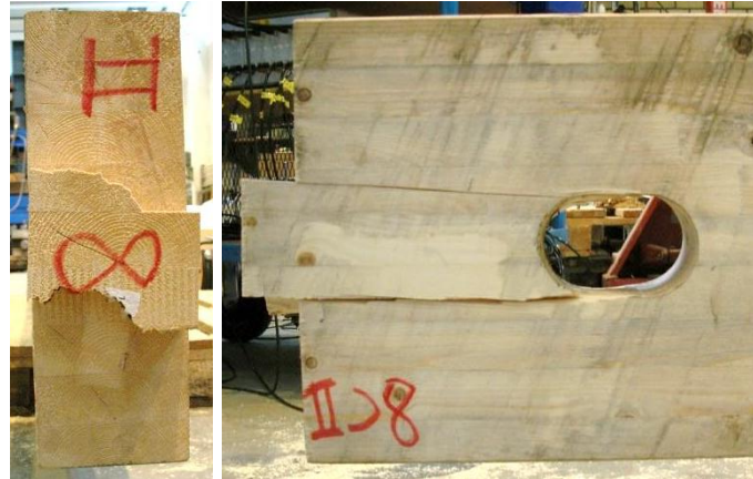
Figure 39 Shear plug in specimen 8.
