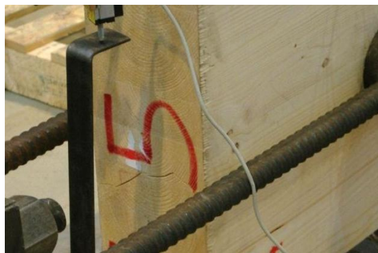
Figure 32 Splitting in specimen 5.
