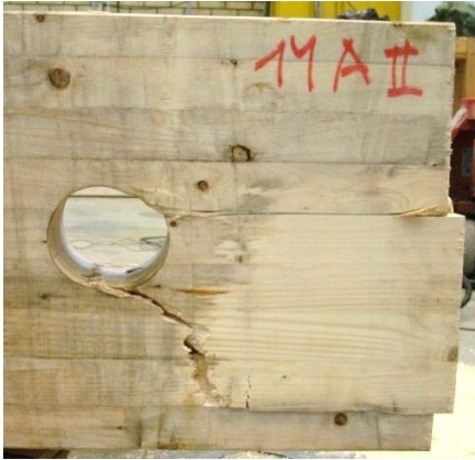
Figure 59 Combined shear and tensile failure in prestressed specimen no. 14.
