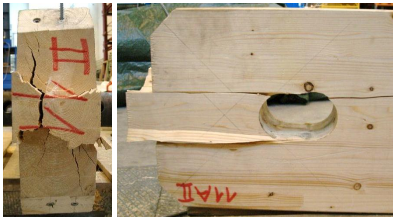
Figure 40 Shear plug in specimen 11.
