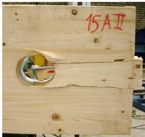
Figure 58 Shear plug in prestressed specimen no. 15.
