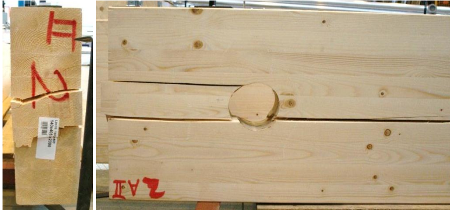
Figure 31 Shear plug in specimen 2.
