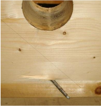
Figure 19 Screw tip appearing on the side (specimen no. 10).
