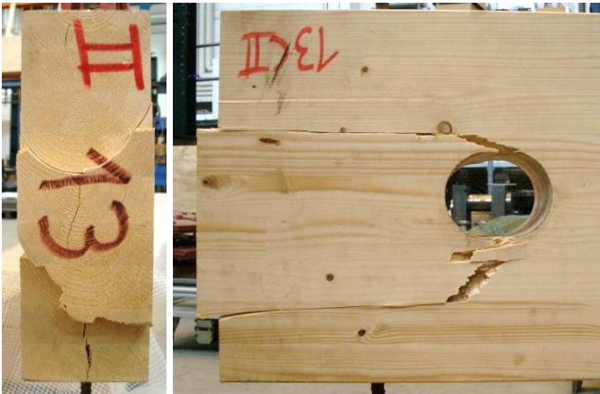
Figure 46 Failure mode in specimen 13.
