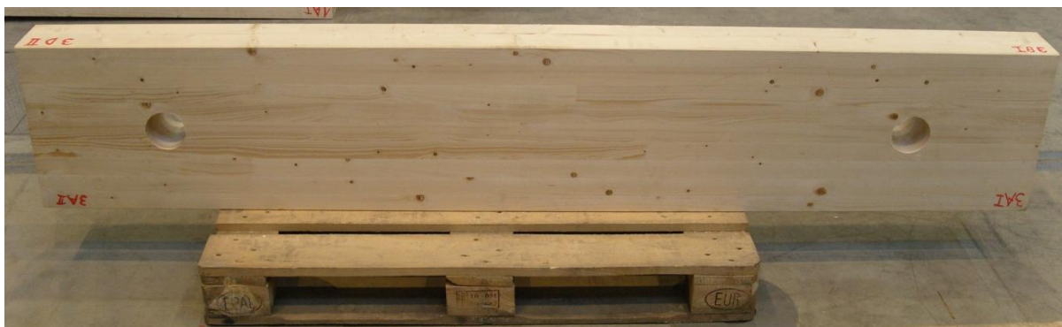
Figure 12 Glulam specimen 140 mm x 405 mm x 2300 mm.
