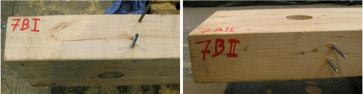
Figure 17 Self-tapping screws in level 0 (specimen no. 7).
