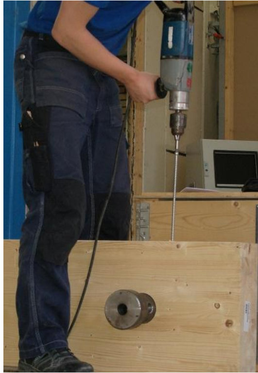
Figure 15 Installing of self-tapping screws.
