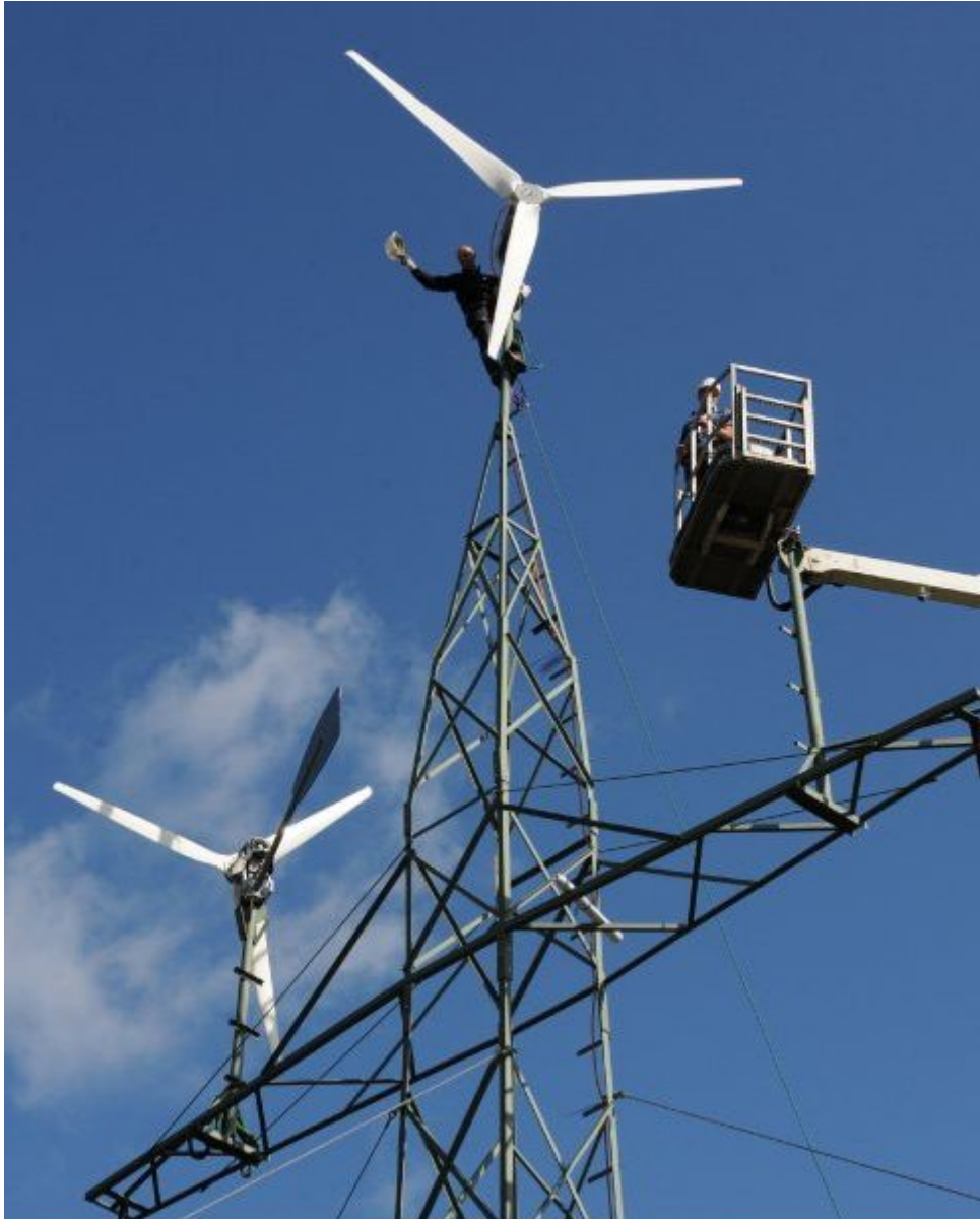
Figure 2.4: Small wind power rotors on power pole (Spiegel Online 2011).
