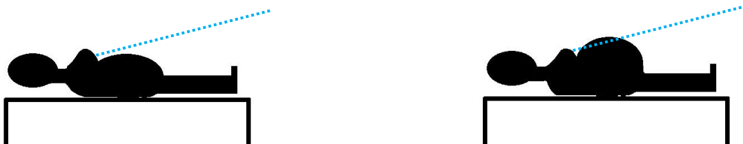
Figure 28. The angle at which the camera is installed in the treatment room ceiling limits the imaging. The first figure is the normal patient case. Shadows could arise above the breast. The second figure shows a patient where the breast will not show at all in the live image due to the large stomach.
