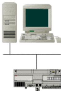
Figure 2.2 A PC running Control Builder and a controller connected via Ethernet.
