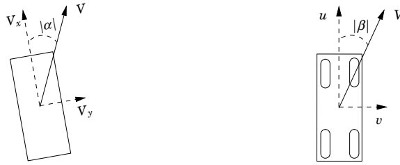
Figure 2.2 Left The tire slip angle. The rectangle illustrates the tire. Right The vehicle side slip angle. The rectangle illustrates the vehicle. Note the difference in scale.
