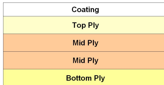
Figure 2.1 An example of a four-layer cartonboard composition.
