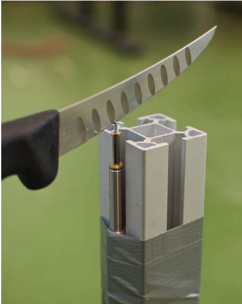
Figure 28: The linear encoder in contact with a knife.
