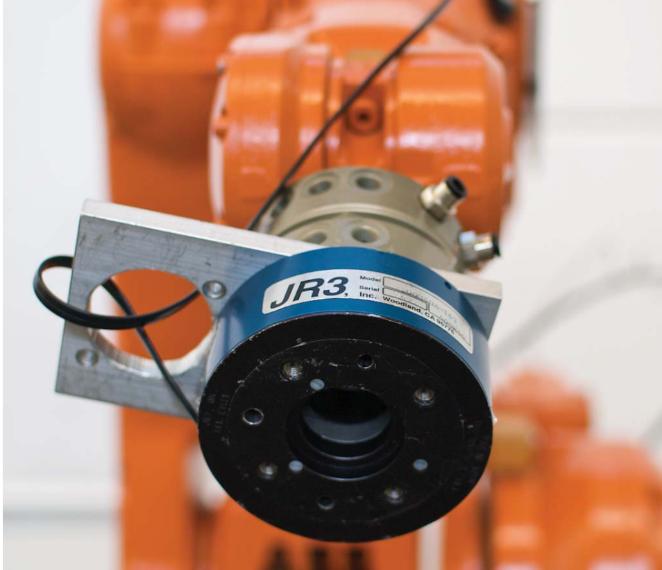
Figure 3: The JR3 force sensor mounted on the robot
