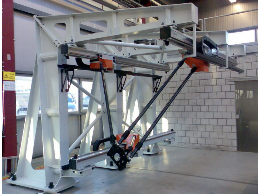
Figure 1.1: New parallel kinematic robot concept developed within the SMERobot TM -project. The carts (red) are controlled in a coordinated way along three rails to move the tool/end-plate along a desired trajectory.
