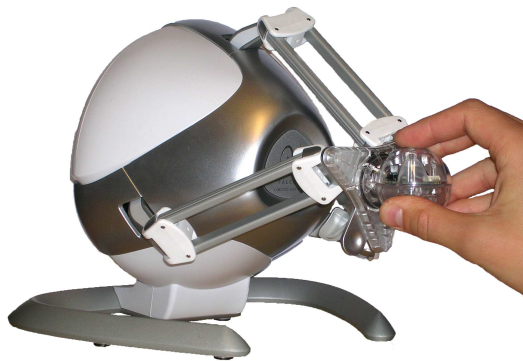
Figure 2.2 The Novint Falcon by Novint Technologies, Inc. is a rather simple haptic device.
