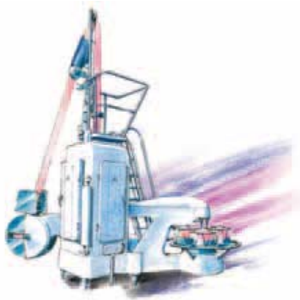
Figure 4.3: One of the first packaging machines for tetrahedron-shaped cartons.
