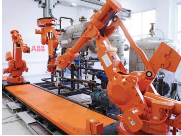
Figure 3.1: All three robots are controlled through an in house system managing path-planning, workstation-robot communications and user interaction.
