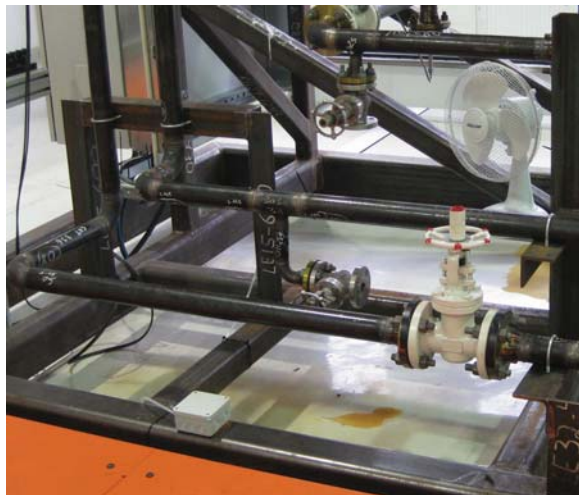
Figure 3.3: The fan was placed inside the process module to let the pipes create realistic turbulence. The white box in the bottom left corner is the release device from where ethanol fumes are ejected.
