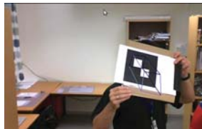
Figure 4.4 The effect of a poorly calibrated camera that can be seen on the cube that OpenGL draws; the lines are not perpendicular to each other
