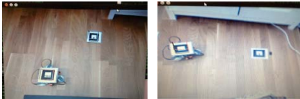
Figure 4.14 (left) Camera 0 showing the mobile NXT-robot moving towards the reference marker, (right) Camera 1 showing the NXT-robot moving towards the reference marker
