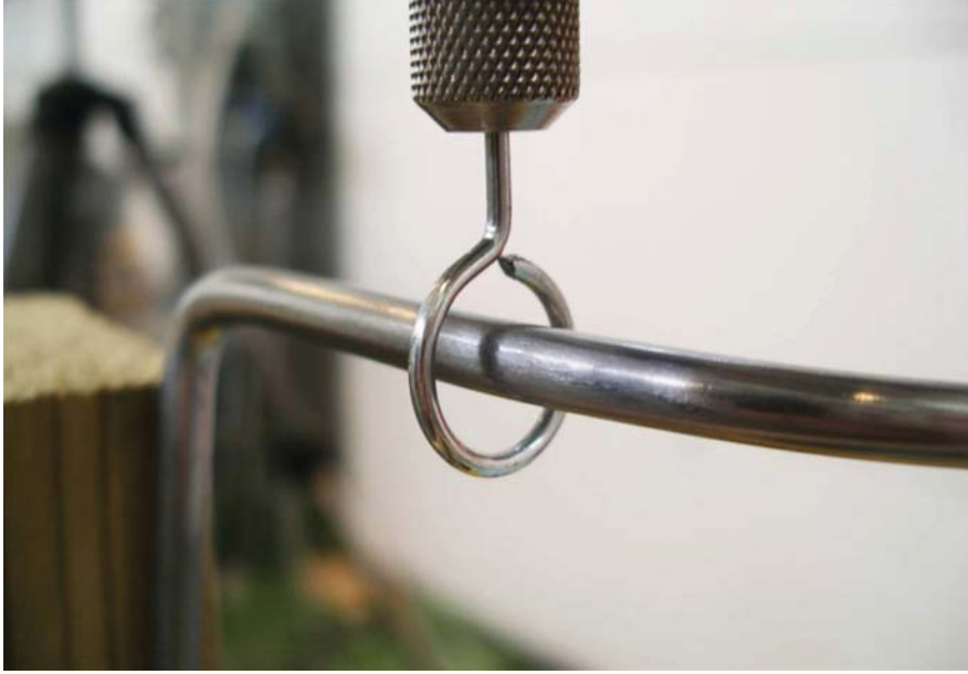
Figure 5.3 In the figure the ring used during experiments with the PVC is shown. The diameter of the ring is 10 mm and the path has a diameter of 5 mm. While traversing the path the ring must not come into contact with the path.
