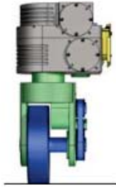
Figure 3.5: The Care-O-bot©3 wheel module [1].
