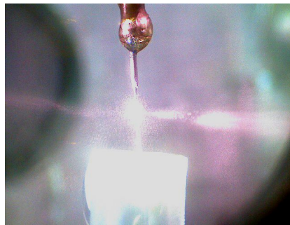
Figure 9: Laser beam focused onto the water-jet inside the vacuum chamber.
