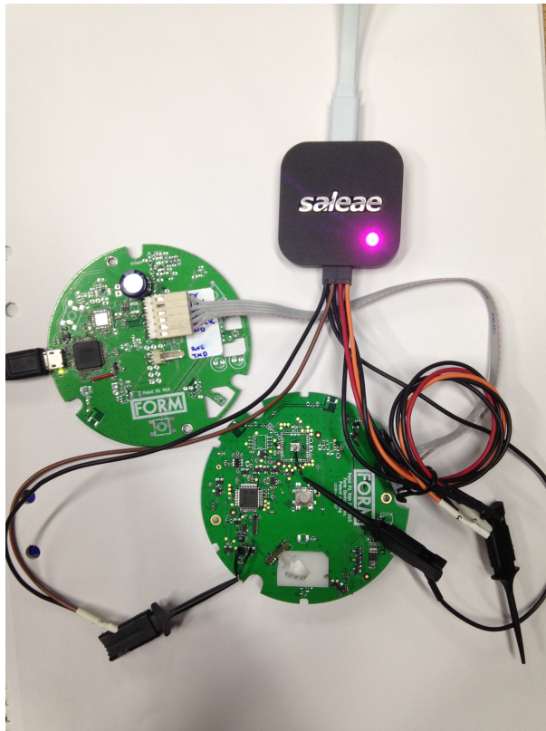
Figure C.1: The debugging setup with a logic analyzer on the I^2C bus.
