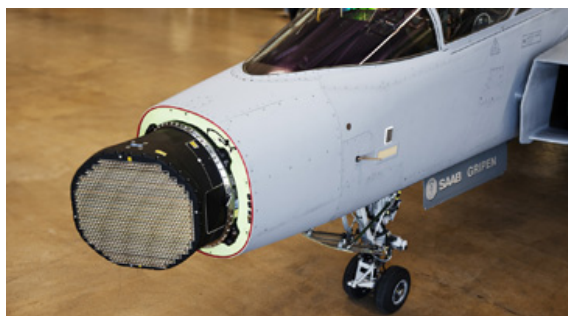
Figure 2: The Raven ES-05 radar mounted on a swashplate on the Gripen E. Figure source: [13]
