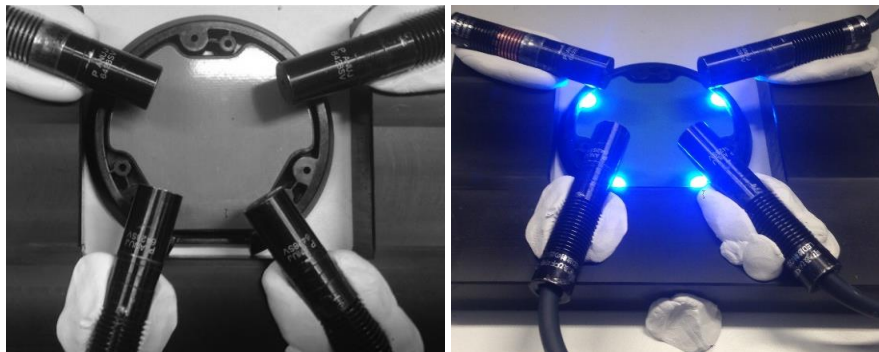
Figure J.2 Fixture with PCB card and UV lamps activated.
