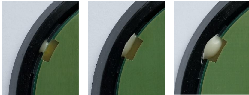
Figure 14.1 Comparison adhesive amount a) 10 mg b) 20 mg c) 30 mg.
