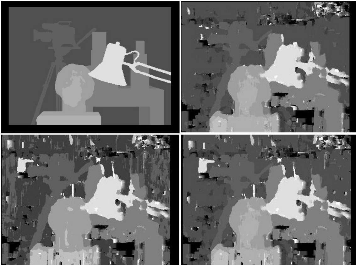
Figure 5.8: 9x9 support window two step disparity check result. Top left: Ground truth; Top right: Without two step; Bottom left: Two step; Bottom right: Two step + Neighbor check
