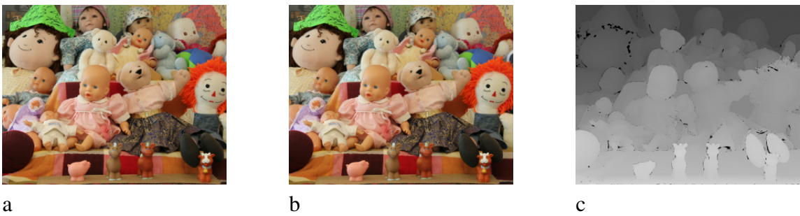
Figure 8.6: Dolls stereo pair and ground truth. a. Left b. Right c. Ground truth
