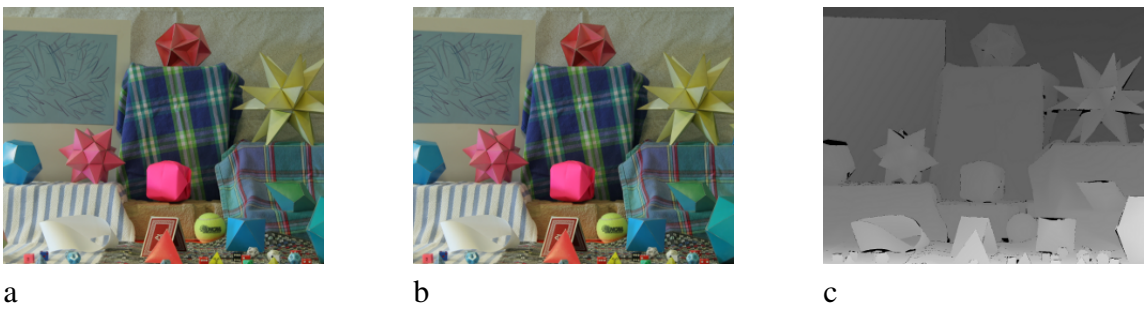
Figure 8.5: Moebius stereo pair and ground truth. a. Left b. Right c. Ground truth
