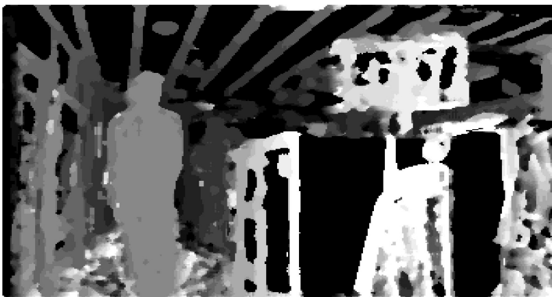
Figure 6.3: Result when using NCC with 5x5 support window size, 0-16 disparity range and uniqueness of maximum control. a, original image b, full window c, sparse window
