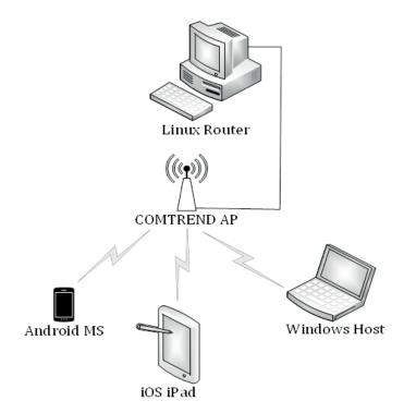
Fig. 41. Implementation setup of the network for the empirical analysis
