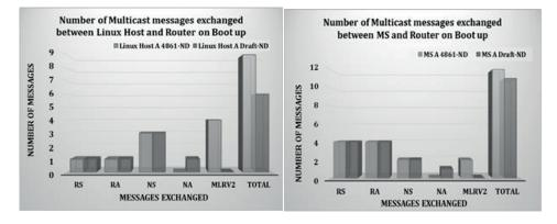
Fig.A.14. Messages exchanged during connection set up for Linux host and Android MS
