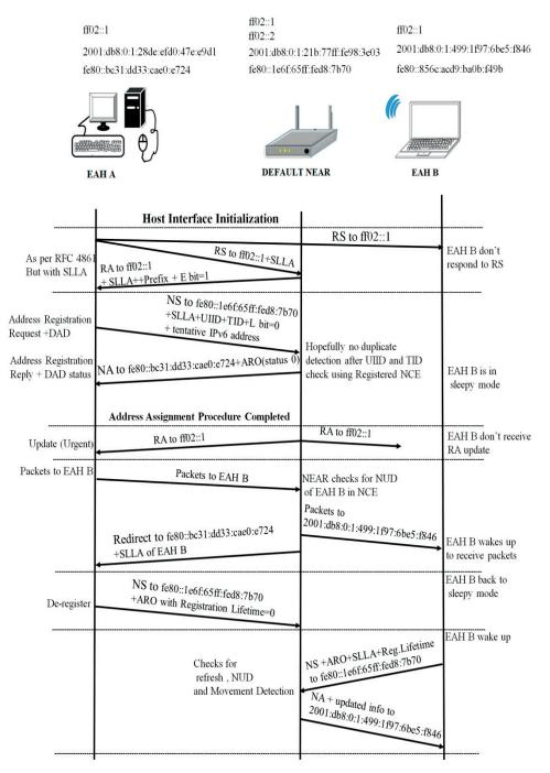
Fig. 22. A signal flow graph of the Address Registration, DAD, Address Assignment, and Refreshing of registration and De-registration procedures according to the efficiency –ND draft
