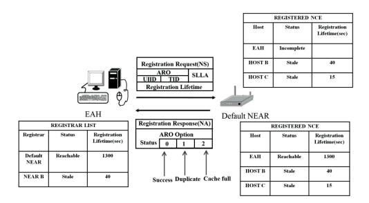
Fig. 21. Address Registration Procedure of EAH
