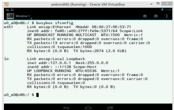
Fig.A.8. Network interface configuration of Android MS in Virtual Box
