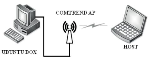
Fig. 25. The implementation setup for RFC 4861 NDP
