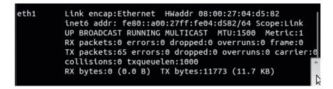
Fig.A.9. Network interface configuration of Router in Virtual Box
