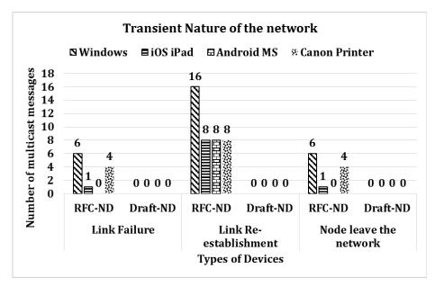
Fig. 52. Multicast messages exchanged during transient nature of the network
