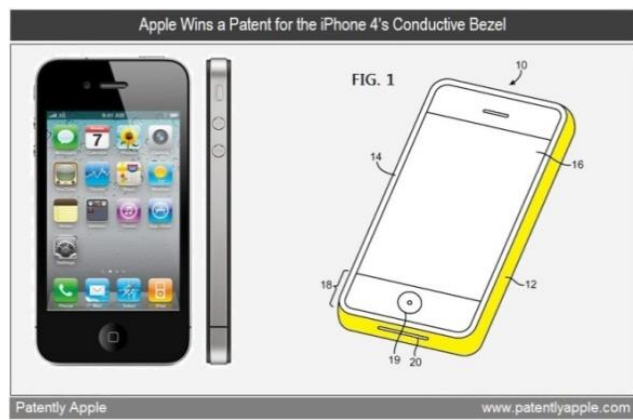
Fig. 3.2: Industrial design of a bezel antenna for Apple iPhone 4
