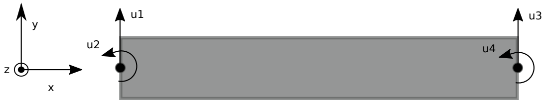
FIGURE 2.2: Degrees of freedom for a beam in the x - y plane.
