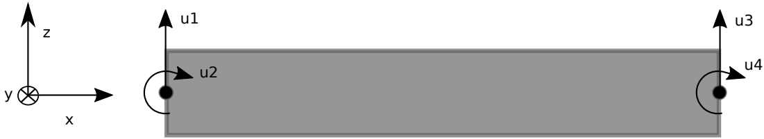
FIGURE 2.3: Degrees of freedom for a beam in the x - z plane.
