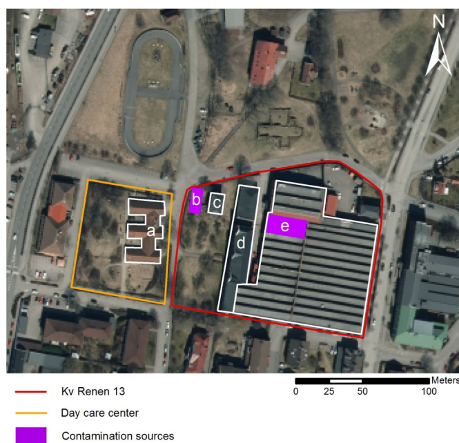
Fig. 2. Overview of Kv Renen 13, with the source areas for the described pollutants and the day care center marked in yellow. a) Day care center, b) sedimentation basin, c) director residence, d) administration building, e) industry building with the cellar marked as contamination sources (© Lantmäteriet I2014/00579).
