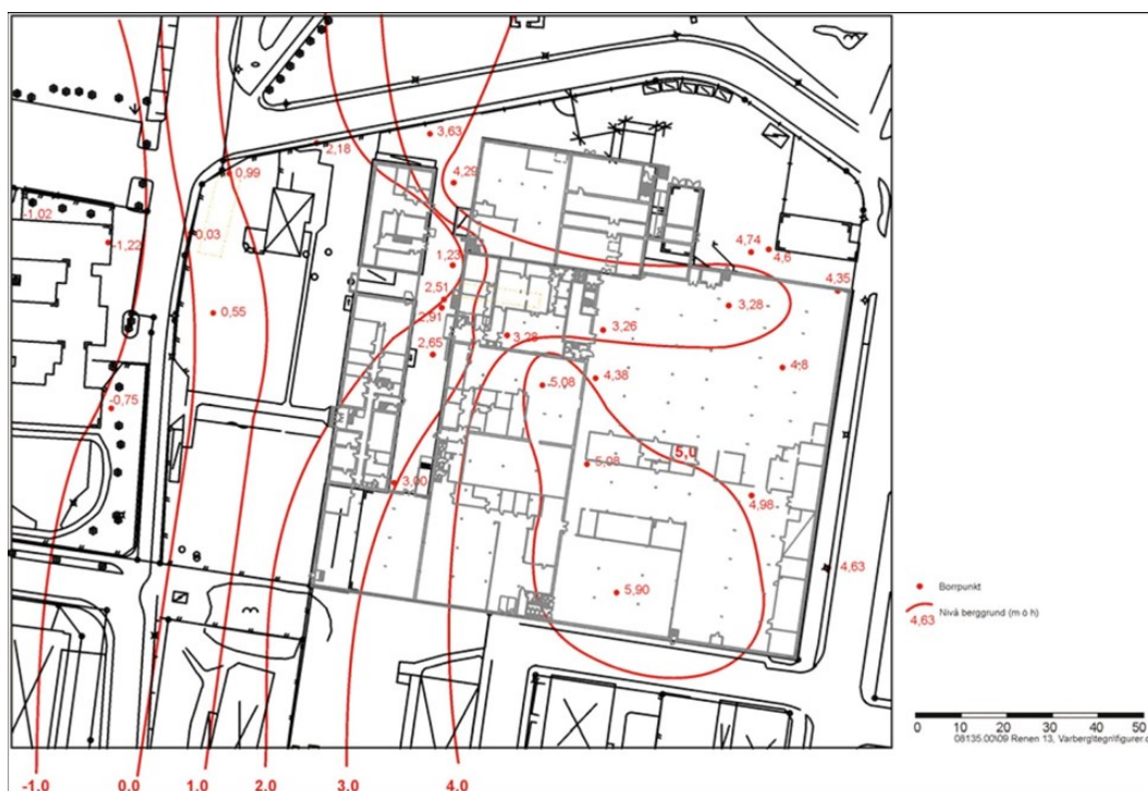
Fig. 5. Investigation of the bedrock location by drilling, and interpolation between the points. The points are given in meters above sea level. The map indicates a dip of the bedrock surface in a westward direction and a lower location in the middle of the estate. Used with permission from Tornberg et al. (2008).
