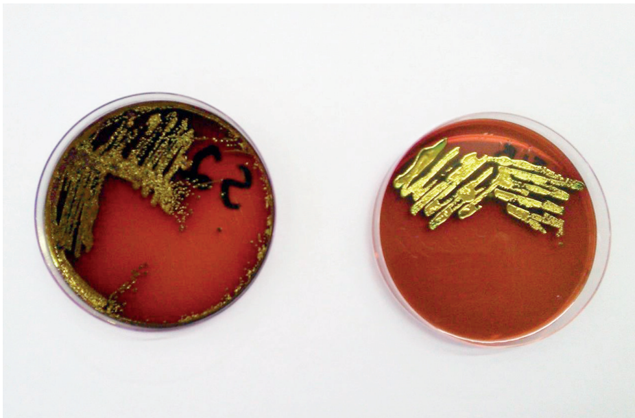
Figure 5.8. EMBA plates for sample S2B to the left and S1B to the right taken from the two different sites in Segoditshane River. The green metallic sheen indicates coliform bacteria.
