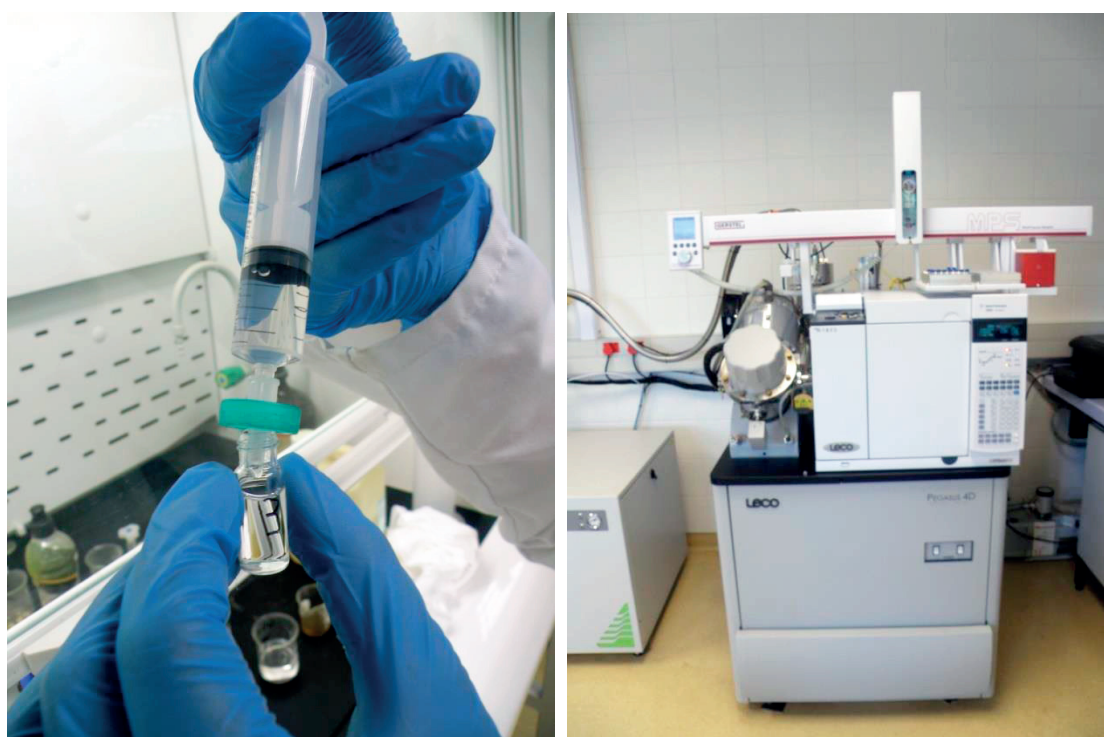
Figure 4.7. to the left and Figure 4.8. to the right.. Filling of the small test tubes with sample to analyse for hydrocarbons in GC TOF MS (Figure 4.7.). Gas Chromatography Time of Flight Mass Spectrometer, GC TOF MS, analyzing several substances in water samples, e.g. hydrocarbons (Figure 4.8.).
