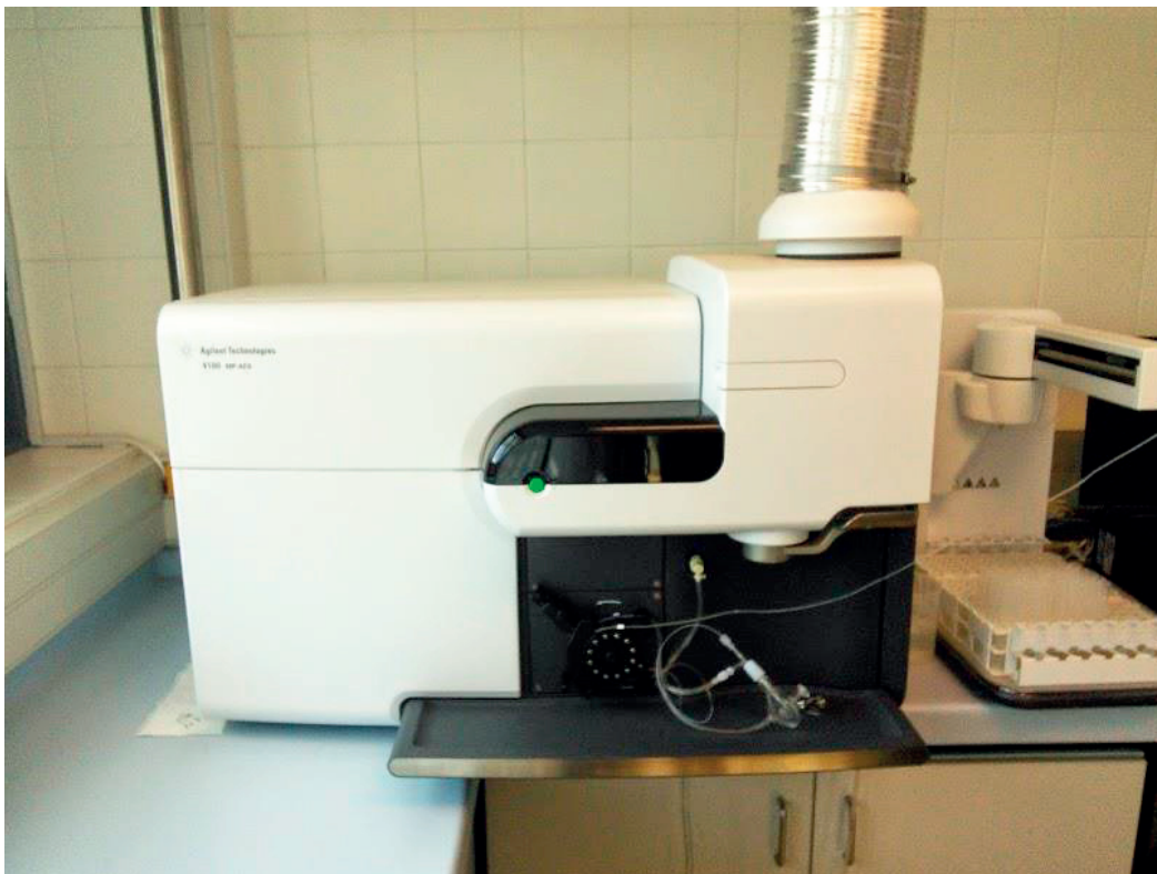
Figure 4.6. Microwave Plasma – Atomic Emission Spectrometer (MP-AES) for analysis of heavy metal.
