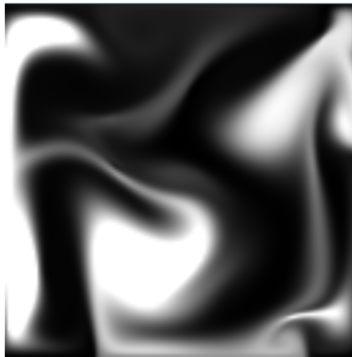
Figure 3.1: Snapshot from a simulation with Stam’s algorithm using a 128 \times 128 grid
