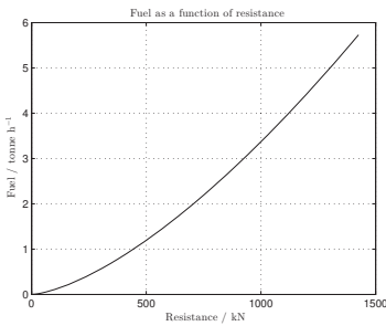
Figure 5.1: Fuel consumption as a function of total resistance.
