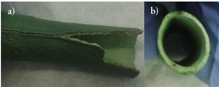
Figure 23. Faults generated to 1 mm tube samples after electrolyte sintering.
