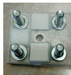
Figure 7. Early setup to create 2 mm thick samples.
