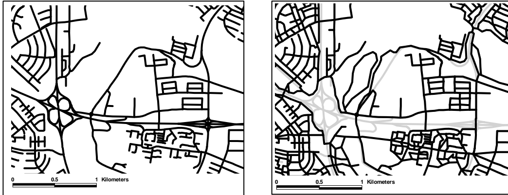
Figure 5.11 Example how the car layer was modified making the bicycle layer. To the left is the original car layer and to the right is the bicycle layer adjusted from the car layer (ArcView maps).
