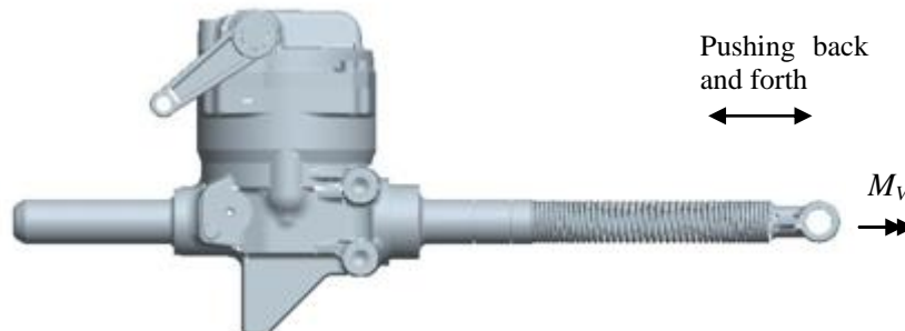
Figure 6.13 Torsional moment of the spindle.
