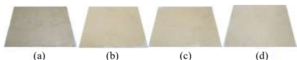
Figure 1. Starch based bioplastics with palm oil concentration of (a). 0% , (b). 2.5%, (c). 5% and (d). 7.5%.
