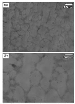
*Figure 2.* (a). Original austenitic ingot optical microgap. (b). The same austenitic optical microgaph from the same sample with the differrent magnification
