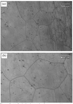
Figure 3. (a) Optical microgaph of new austenitic sampel after homogenization at 1200 °C for 20 h. (b). The same optical microgaph of new austenitic sampel after homogenization at 1200 °C for 20 h, with the differente magnification.
