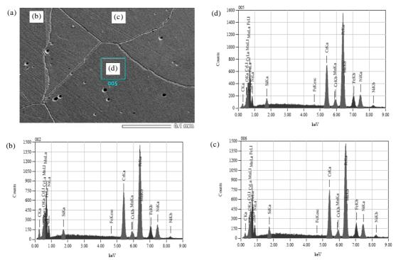
*Figure 4.* SEM micrograph and the supplemental EDS results: a. Microstructure of A1 ingot sample; Here it is clearly shown that the surface is relatively homogenous with a minor part of the surface showing a grey colour covering a narrow area on the left hand side bordered by the irregular line running from top to bottom; b. EDS results from a narrow but long top to bottom region c. EDS results from a homogenous region at the top. d. EDS results from the central region.
