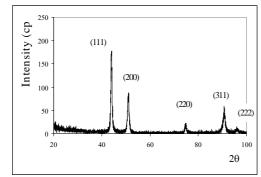
Figure 5. A1 austenitic material X-ray diffraction pattern shows the fcc crystal structure
