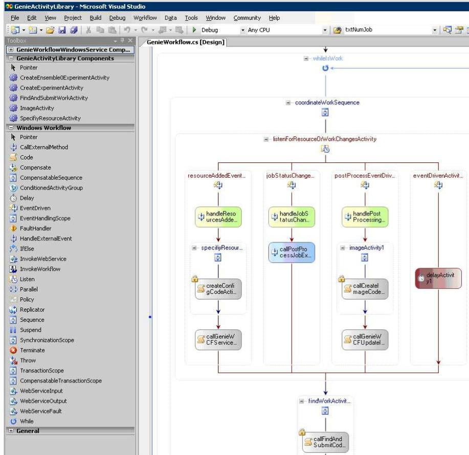
**Figure 2:** Design of the GENIE workflow in the WF Designer with Visual Studio
