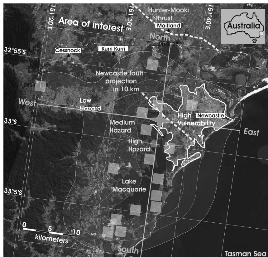
Figure 4. Hazard map of potential coal mining–triggered earthquakes in an area of the Newcastle coalfield in New South Wales (Australia). The squares show the locations of underground coalmines in approx. 500m depth. The resulting stress changes in the Earth’s crust are qualitatively indicated by the labels “Low Hazard,” “Medium Hazard,” and “High Hazard.” The projection of the fault that ruptured during the 1989 M5.6 Newcastle earthquake (star) in about 10km depth intersects with the area of high and medium earthquake hazard. Furthermore, the urbanized area of the city of Newcastle (“High Vulnerability”) also coincides with the area of medium and high hazard. This indicates why the Newcastle earthquake had such high impacts on the human security [23, 4].
