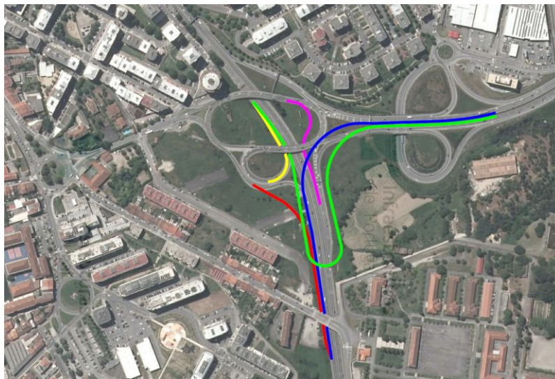
Figure 8: Proposed infrastructure additions Alternative 3
