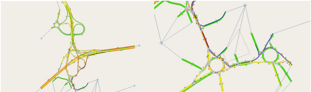
Figure 35: Map based outputs showing flow density in different sections with color coding
