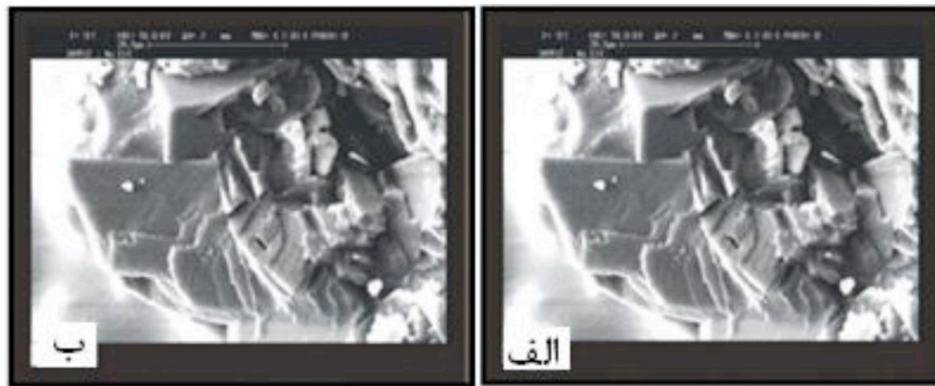
Figure 3: Scanning electron microscopy image: a) Planner-s dolomite crystal (scale 20 \mu ); b) Planner-e dolomite crystal (scale 10 \mu )
