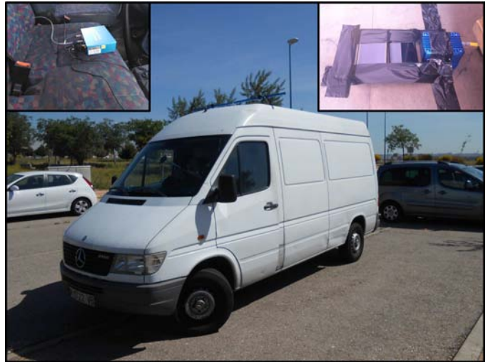
Fig. 1. Vehicle used in tests equipped with two smartphones: Samsung Galaxy S8 and Xiaomi Redmi 3; and the VBOX IMU connected with the VBOX 3i data logger of Racelogic
