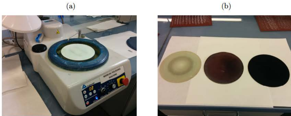
Fig. 3.2: Polishing equipment and accessories: (a) Manual polishing machine; (b) Main polishing clothes: MD-Mol, MD-Nap and MD-Chem (from left to right).
