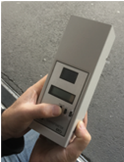
Figure 1: EKO handheld sunphotometer, the last handheld sunphotometer used at Cape Grim.
