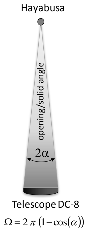
Fig. 10 Illustration of the solid angle for propagation of Hayabusa radiation to the DC-8.
