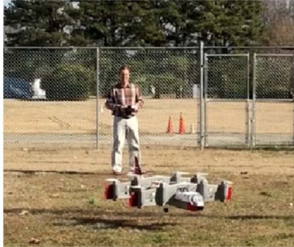
Figure 26. LA-7 CERTAIN Net Hover Flight Testing
