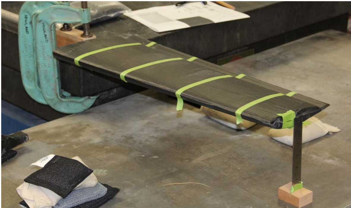
Figure 22. Foam Core Carbon Fiber Forward Wing Load Test Article
