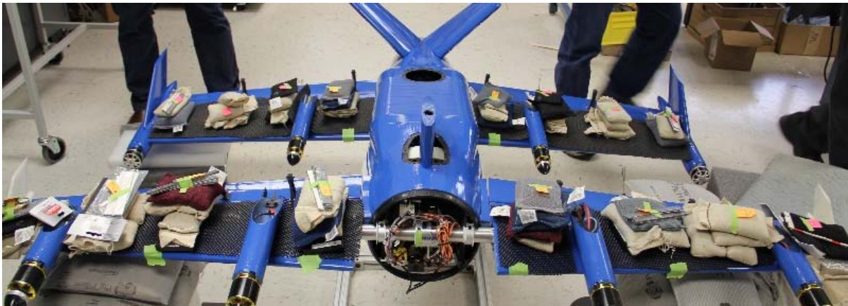
Figure 46. LA-8 65lb 3G Load Test
