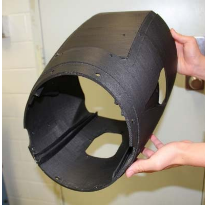
Figure 14. FDM Nylon 12 Fuselage Section
