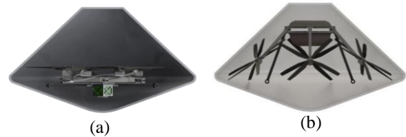
Figure 2. Hexacopter configurations: (a) four-bladed rotating, (b) four-bladed hinged.
