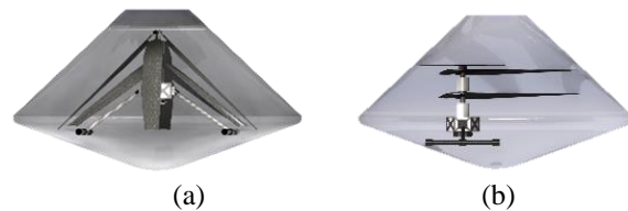
Figure 3. Coaxial configurations: (a) four-bladed, drooped, (b) three-bladed, in-plane folding.
