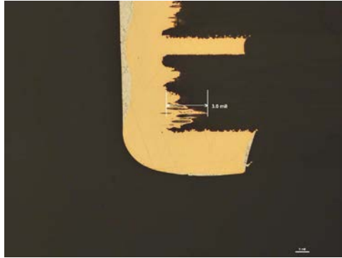
Copper wicking in excess of 2.0 mil
